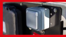
Socket with differential circuit breaker Equipment can be plugged into the basket.
