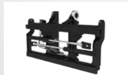
2.540 mm wide Hook Type Dual Function carriage with Side Shift and Fork Positioner (FP can be as independent or simultaneously acting)
