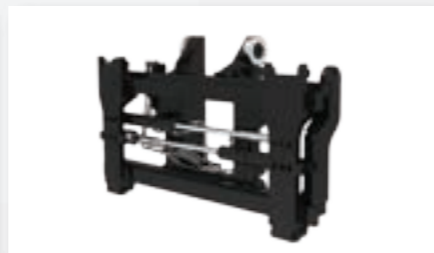
2.540 mm wide Hook Type Dual Function carriage with Side Shift and Fork Positioner for Quick Disconnect forks (FP can be as independent or simultaneously acting)
